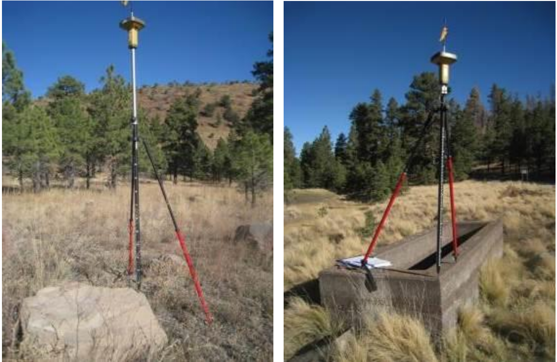
Figure 2.11 Example of a natural feature (boulder; left) and a man-made feature (trough; right). The features were measured in the field then located on the images to be used as GCPs.
