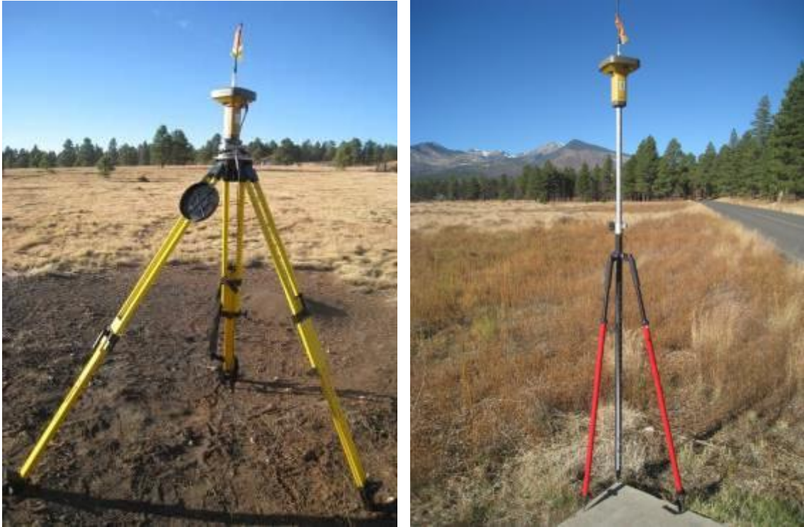
Figure 2.10 The base (left) and rover (right) receivers used to determine coordinates of additional GCPs in the field.
