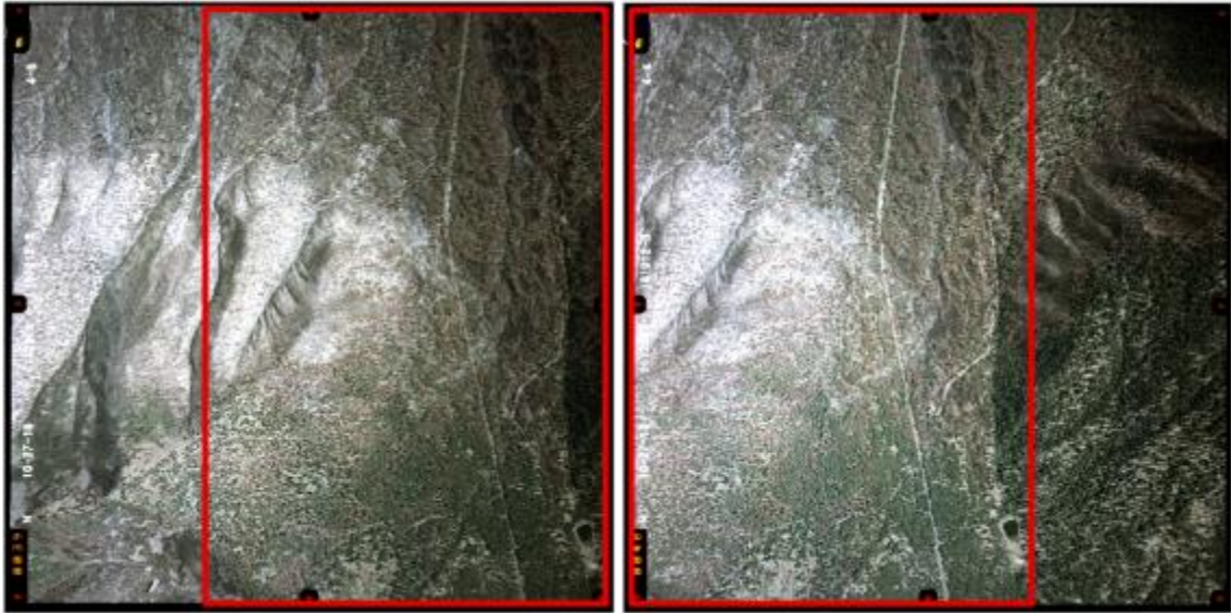
Figure 3.2 Image 0405 (left) and 0404 (right). The red boxes indicate the overlap (approximately 70%) between these two images. These images were chosen based on the high number of GCPs found in the overlap area. Note: Top of image is east.
