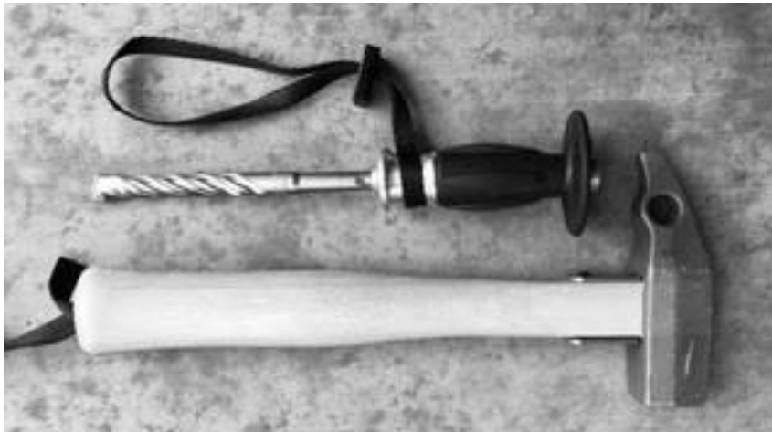
Figure 1. Tools Used for Hand Drilling: A hand drill and hammer
