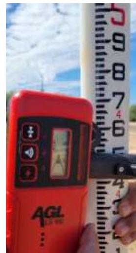
*Figure 13: Laser Receiver Calibration*
