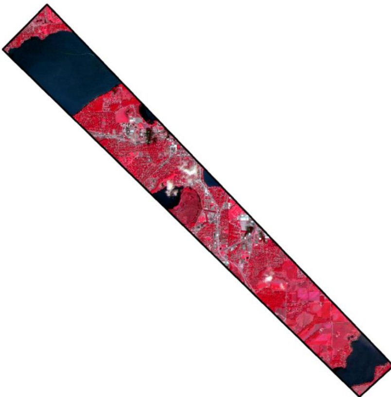
Figure 7: Clipped raster with Nearest Neighbor resampling and Color Infrared band combination.
