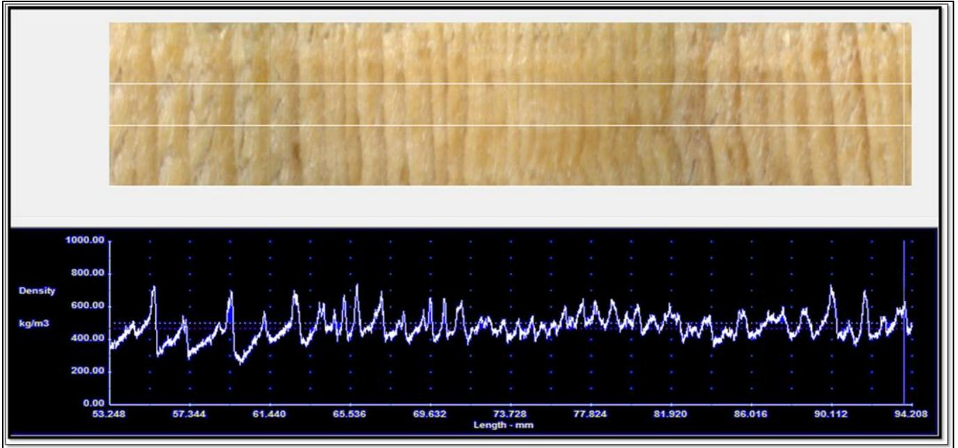
**Figure A5:** A sample readout from the QTRS-01X Tree Ring Scanner X-ray densitometer. A photograph of the wood sample accompanies the pith-to-bark density profile. Peaks and valleys in the readout indicate spikes and drops in wood density correlated with latewood and earlywood bands across the annual rings.
