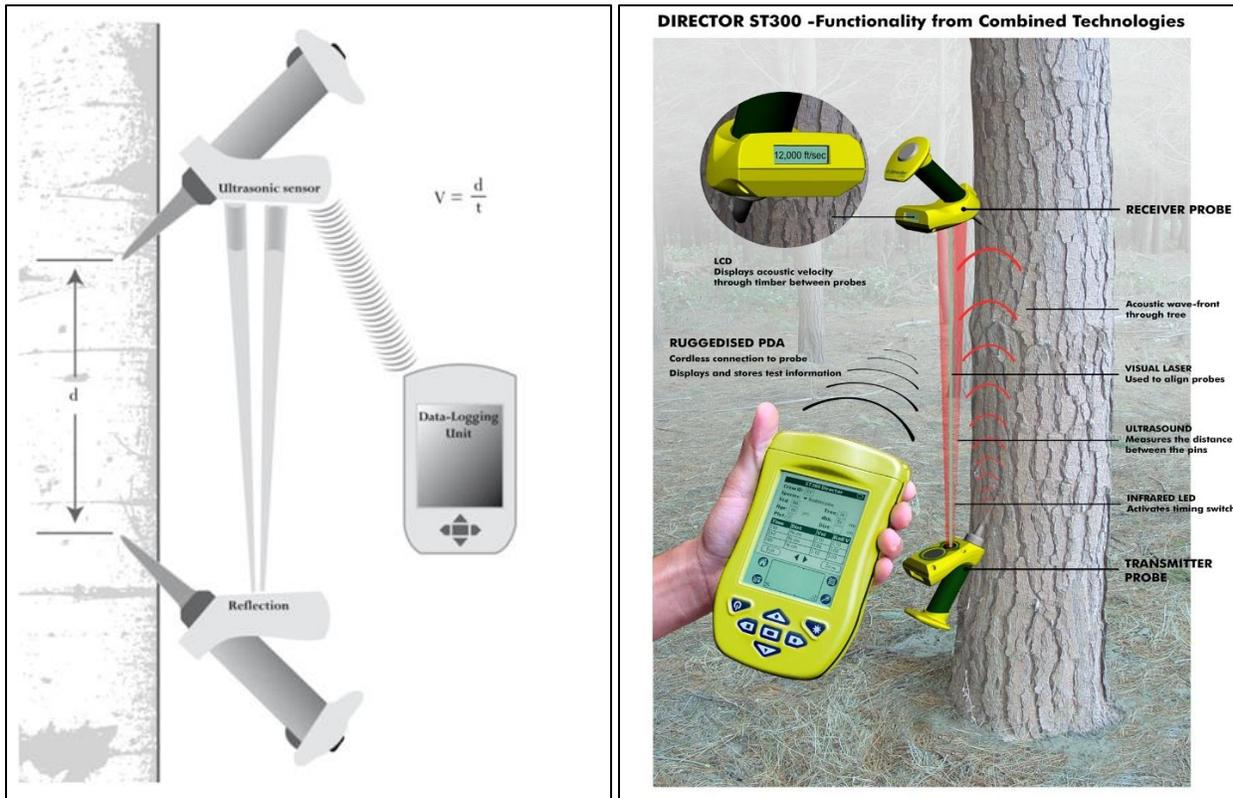
**Figure A3:** Diagrams of the ST300 operating principles (left) and operating system (right). An acoustic wave produced by a specialized hammer travels between the lower and upper probes of the ST300 Hitman acoustic tool. The transit-time of the wave between the two probes is recorded and velocity calculated in miles per second and stored on a portable data logger. Photo credit: Paradis et al 2013, Fibre-gen.
