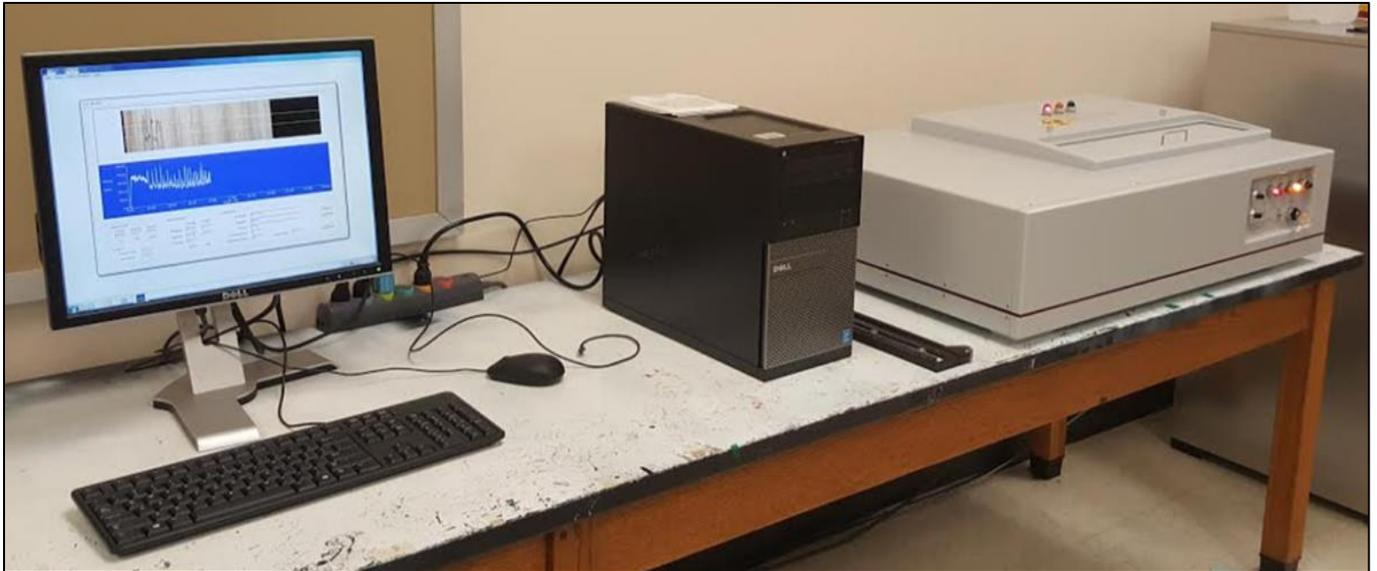
**Figure A4:** The Quintek QTRS-01X Tree Ring Scanner scanning and recording the wood density profile of a ponderosa pine sample.
