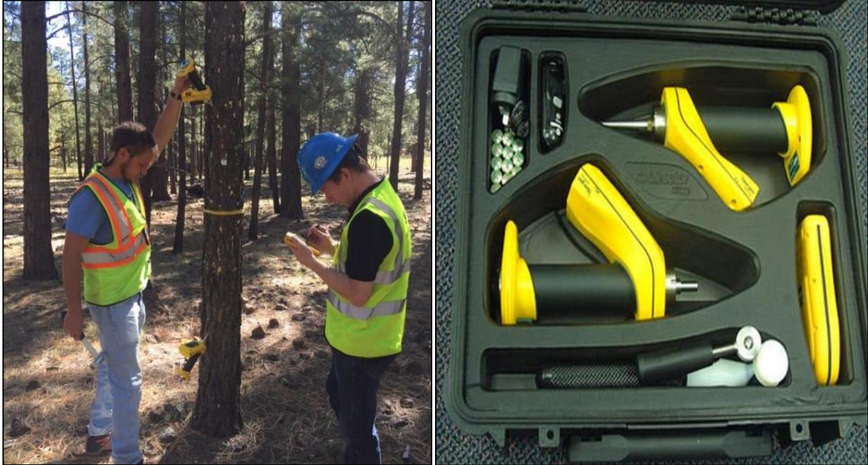
**Figure A2:** The ST300 Hitman in use at the Centennial Forest experimental site (left); the ST300 Hitman acoustic measurement tool (right). Photo credit: Fibre-gen.
