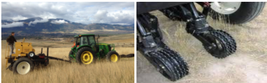
Figure 8. A tractor pulled a seed drill (left) and imprinter (right).
