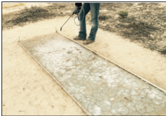
Figure 10. Addition of polyacrylamide to experimental plot. Photo credit: A. Faist.
