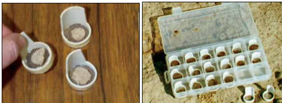
Figure 13. Soil aggregates on slake kit strainers made from PVC pipe and wire mesh (left) and a complete slake kit with 18 soil aggregates ready for evaluation (right). Photo credit NRCS.
