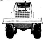
Tree Farmer model C5B features 97 HP diesel economy; %" armour plate construction; high ground clearance; four wheel drive; excellent operator visibility; centre hinged frame; solid oscillating front axle; and a broad selection of attachments and options.
