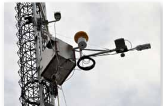
The array of sensors used to measure carbon dioxide, water vapor, windspeed and other environmental conditions.
